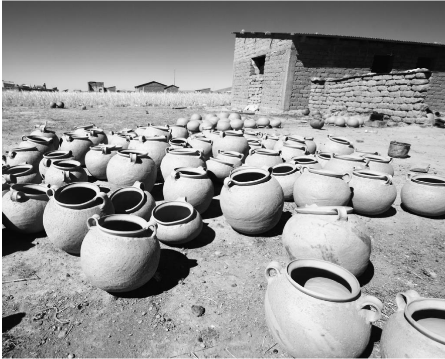
Bolivian Pottery drying prior to firing (left), the ceramic life cycle from Sillar and Tite (2000) (right).
